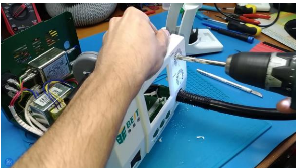
16. Drill final holes with 7mm drill bit
